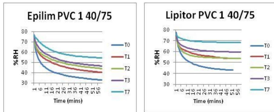
Figure 2. Moisture profiles of Epilim and Lipitor Tablets packed in 250 PVC Clear and stored at 40°C/75% RH
