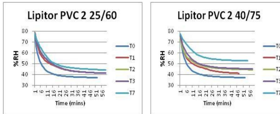
Figure 4. Moisture profiles Lipitor Tablets packed in 250PVC/60PvDC Opaque and stored at 25°C/60% RH and 40°C/75% RH
