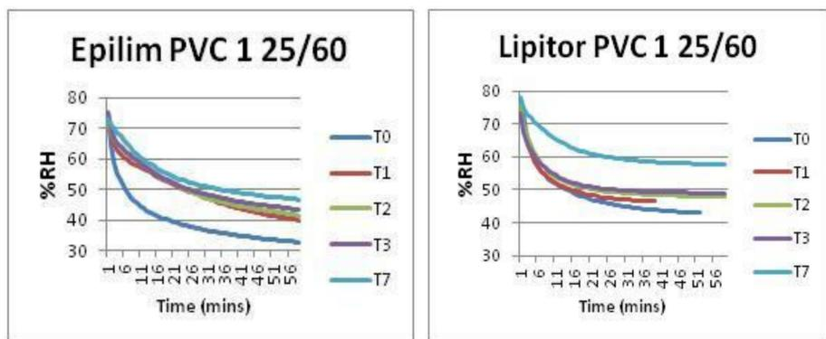
Figure 1. Moisture profiles of Epilim and Lipitor Tablets packed in 250 PVC Clear and stored at 25°C/60% RH
